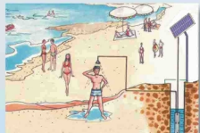
Water supply for small showers on the beach
